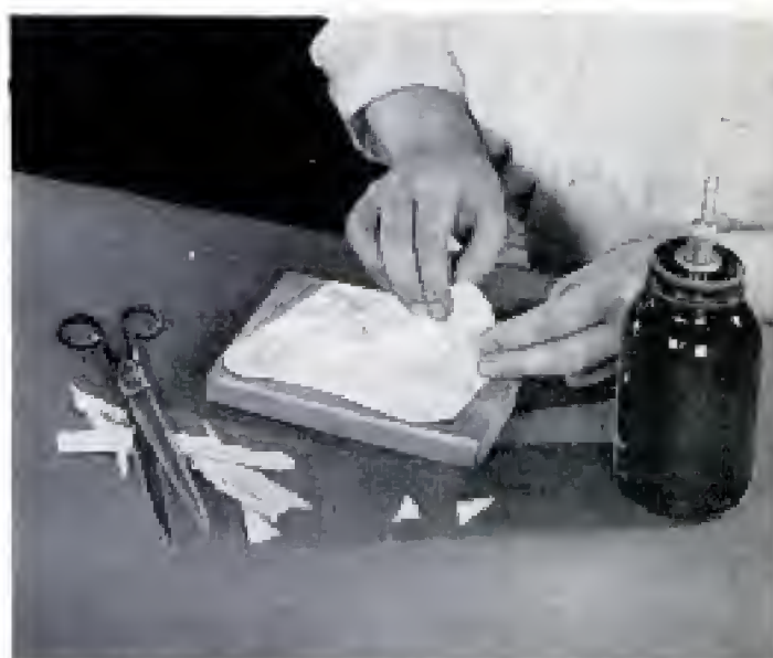
Above, using rubber cement, the finished printing plate is mounted on a wooden block. Below, after inking with linoleum-block ink, the printing block is used like a regular rubber stamp to reproduce the original design
